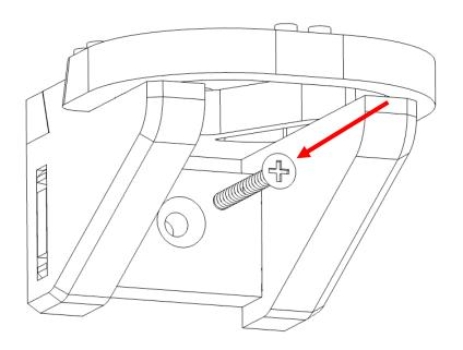
Use the provided wall fixings to secure to the wall. Do not over tighten the screws (use a screwdriver only).
